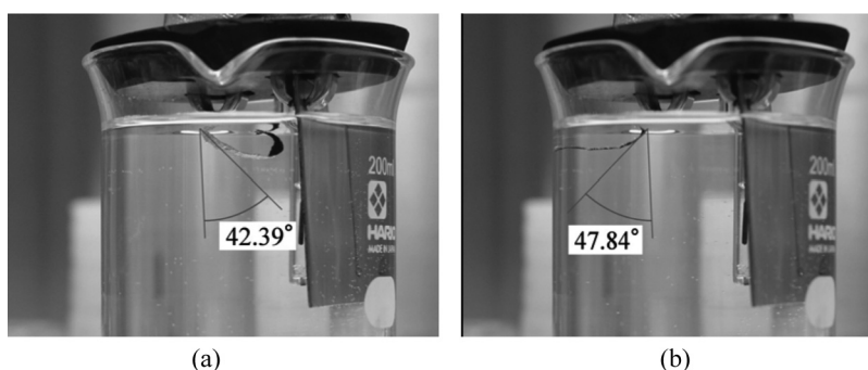
Figure 3. Bi-directional bending organic actuator of PPy1 ( 68.8 \mu\text{m} )/adhesive tape.
